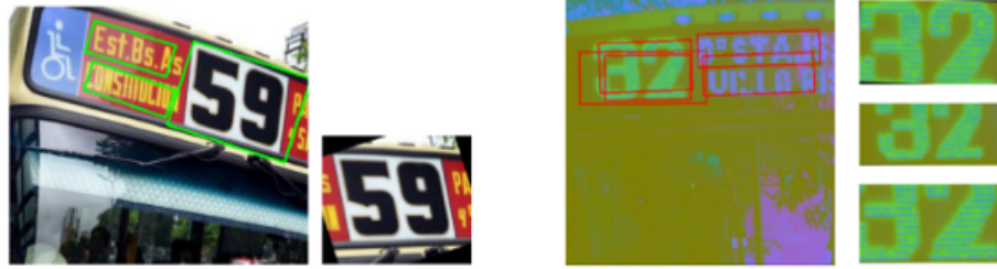
Fig. 4. Detection by EAST using: confidence : 0.5 and IoU : 0.6. (To the left: Buenos Aires's bus - 'rgb' transformation - vinyl number. To the right: Córdoba's bus - 'yuv' transformation - number formed by LED diodes and partial detections).
